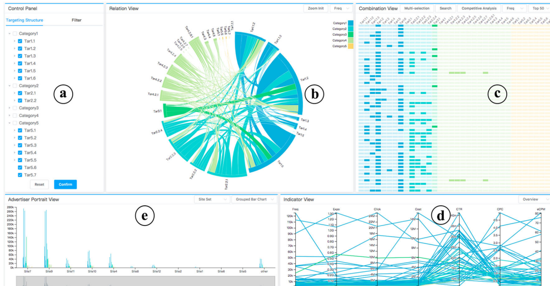
Fig. 1 The user interface of TargetingVis. a Control Panel allows users to adjust the structure of targeting or filter the data to change other linked views, b Relation View summarizes the relations in hierarchical data to discover targeting usage and disclose problems in the design of targeting structure, c Combination View shows targeting combination patterns generated by advertiser delivery behavior so that users can find useful combinations and avoid abnormal combinations, d Indicator View demonstrates the overview and detail indicators corresponding to the targeting combination pattern to help users determine the quality of a combination, e Advertiser Portrait View displays the concrete performance of advertiser delivery behavior in different dimensions and indicators
